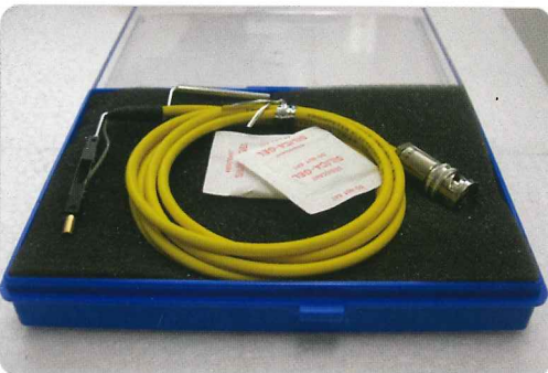
Probe arm with Triaxial cable
