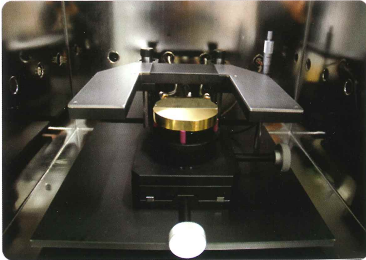
Probe station and chamber inside
