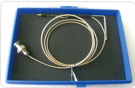
Probe arm with BNC cable
